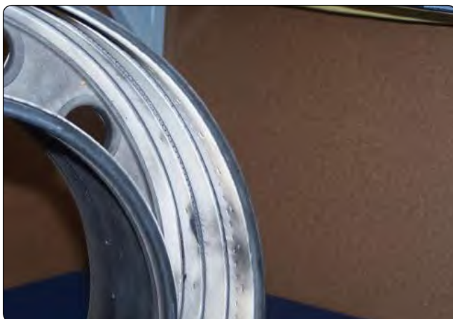
Figure 1-55. Annular combustion chamber liner.
