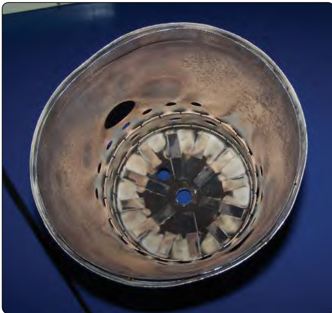
Figure 1-53. Inside view of a combustion chamber liner.
