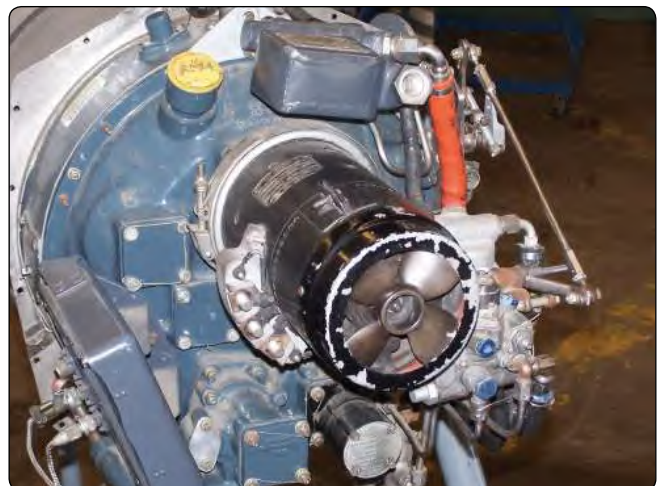
Figure 1-45. Typical turboprop accessory case.
